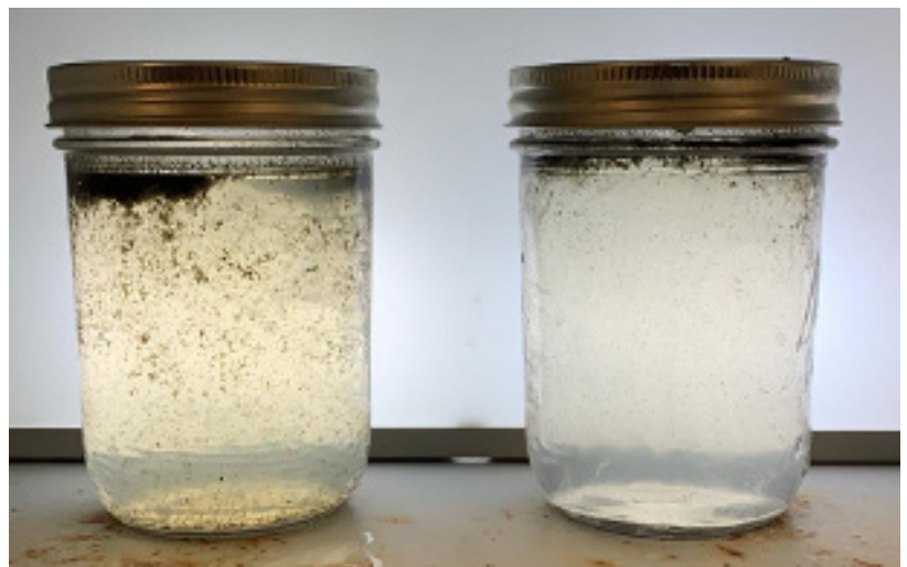
Figure 1: Floc tube samples LEFT: Sample of the flocculated influent pre NanoNet Fe™ RIGHT: Post NanoNet Fe
